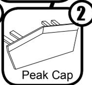
**1** Slide **Peak Cap** legs under **Ridge Cap** and secure **Ridge Cap** ends with four **Small Bolts and Nuts** on each end as shown.
