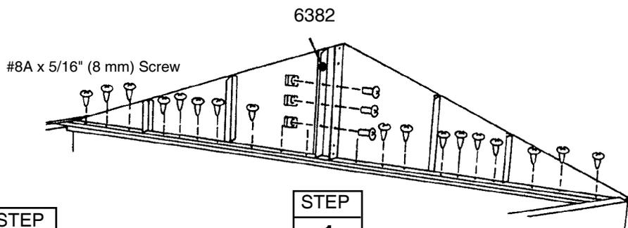
NOTE: For rear entry door installation only use 3/32" dia. drill to clear gable holes through rear frame into track.
