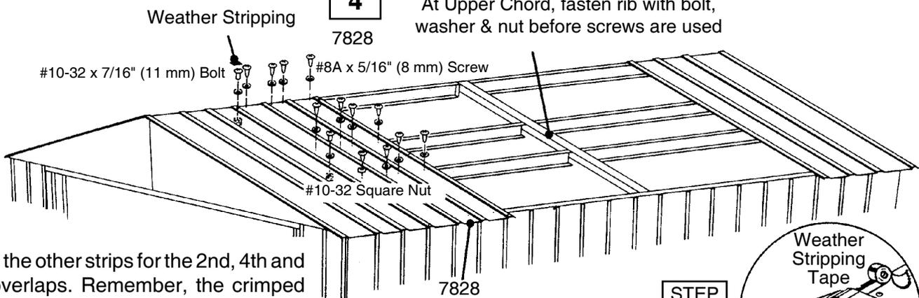
Save the other strips for the 2nd, 4th and 5th overlaps. Remember, the crimped rib is always overlapped by wide rib of adjacent panel. Repeat procedure with 2 more middle roof panels working side to side.
