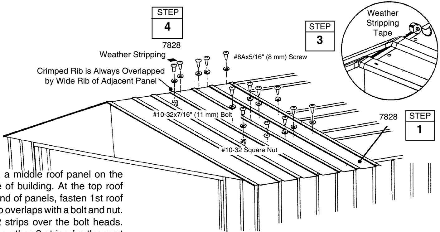
**4** Install a middle roof panel on the left side of building. At the top roof beam end of panels, fasten 1st roof panel rib overlaps with a bolt and nut. Press 2 strips over the bolt heads. Save the other 2 strips for the next overlap. Remember, the crimped rib is always overlapped by wide rib of adjacent panel.
