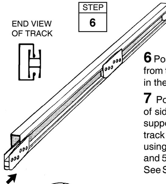
**6** Position **door slides** onto the legs, from the end of door track, as shown in the end view.
