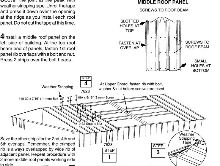
2 more middle roof panels working side to side. Î 5 MIDDLE ROOF PANELS Î LEFT ROOF PANEL **RIGHT ROOF PANEL** FRONT 占 REAR 1ST 2ND 4TH 5TH 33
