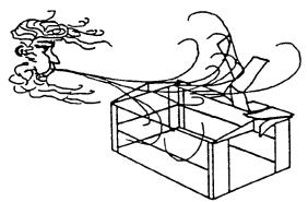
•Do not attempt to assemble the building on a windy day, because the large panels acting as a "sail", can be whipped about by the wind making construction difficult and unsafe.
